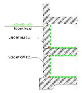
joint. Fill the opening with VELOSIT RM 211 and finish with VELOSIT CW 111.
